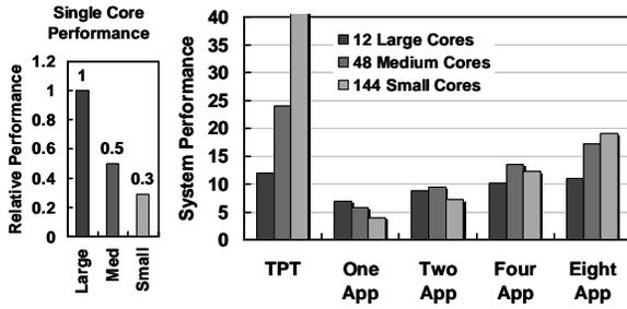
Figure 6: Performance of Large, Medium, and Small Cores
